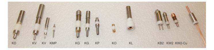
Mineral insulated (MI) cables require due to their special construction a special type of end contact sealing the cable. Due to the hygroscopic insulation material (MgO, Al2O3, SiO2) between current-carrying inner conductor and metallic sheath make it necessary to perform a excellent sealing of cable ends from the surrounding atmosphere.
